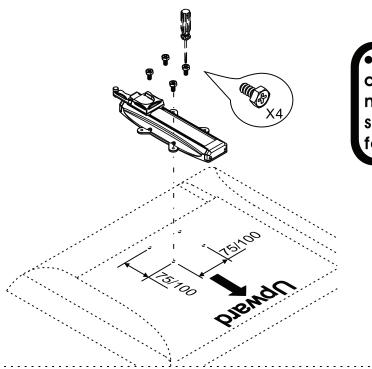
•These screws (M4/15L) are just for special monitor when the original screws are too short to fasten.
